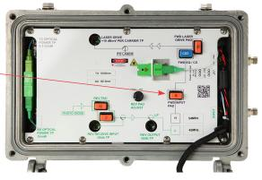
**Note** – For Optimal SNR/MER do not pad here on first stage unless the TIP is > 20 dBmV. For Up Sloped Inputs approximate or calculate Total Composite Power. A few Channels at 22 dBmV at the end of the spectrum with a 12 slope will not require 2 dB Pad.
