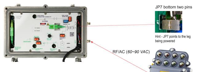
Powering the AIFA via Antronix Milenium Series SDPE Power Passing Multi-Taps
