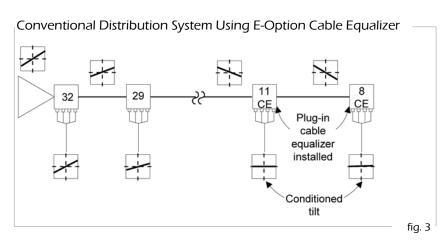
The cable equalizer is a full-bandwidth equalizer from 5 to 1002 MHz. Cable equalizers have more attenuation at the lower frequencies and therefore, allow the cable modem to transmit at a higher level, while attenuating the ingress and noise generated at the customers' premises. This results in an increased carrier to noise/ingress ratio.
