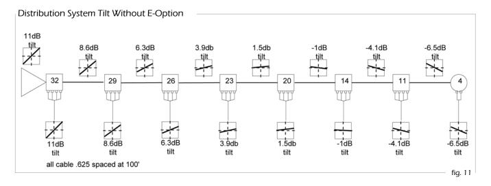
Adding E-Option plug-in cable simulators (CS) at the high tap value locations and cable equalizers (CE) at the low value tap locations the tilt can be controlled to meet any design specifications. The traditional design has a +11/-6.5dB tilt while the E-Option design maintains ±2dB tilt throughout the distribution system (see fig.12).
