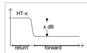
**High Pass Filter (HP):** The high pass filter is used to eliminate ingress generated from the subscriber premise from entering the system. The advantages of the high pass filter are:
