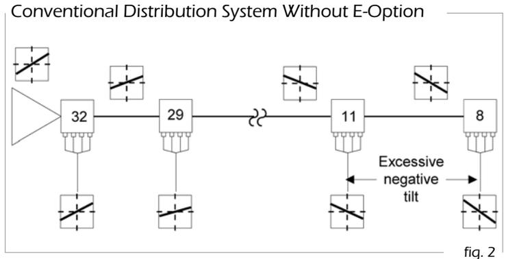
The resultant tilt can cause problems with set-top converters, which can have tight input level and tilt requirements. To overcome this problem the E-Option tap has plug-in cable equalizers available in several values to provide the optimum tilt for each location (see fig. 3). By equalizing at each tap location you can extend your distribution line further without adding additional expensive amplifiers or inline equalizers to control the tilt.
