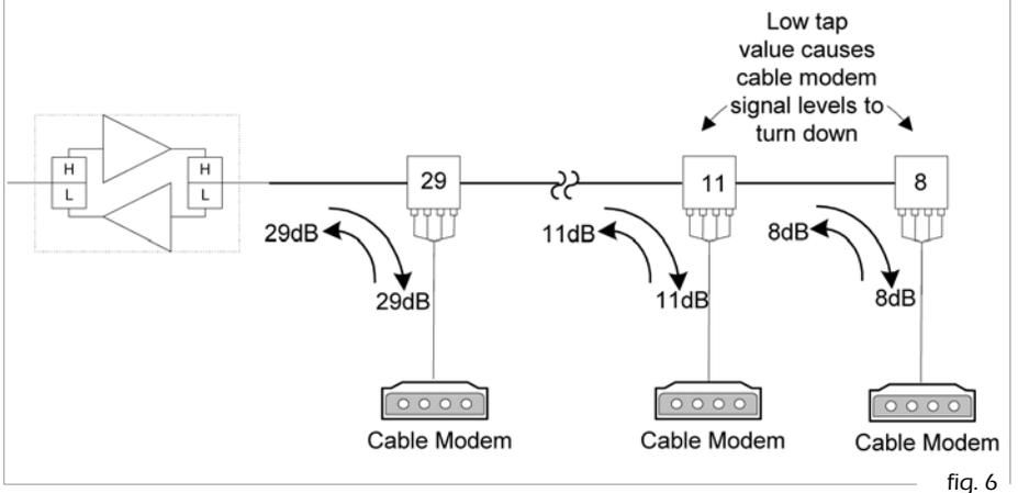
Conventional Distribution System Using Cable Modems With E-Option Return Path Attenuation
