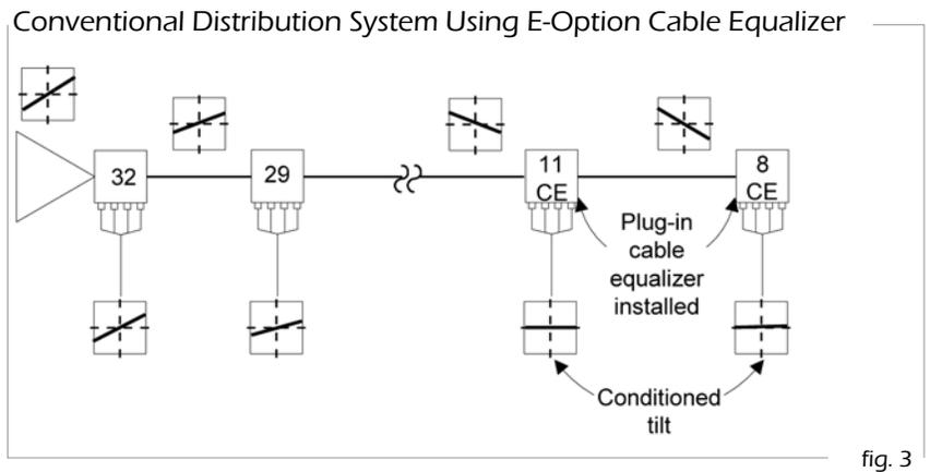
The cable equalizer is a full-bandwidth equalizer from 5 to 1002 MHz. Cable equalizers have more attenuation at the lower frequencies and therefore, allow the cable modem to transmit at a higher level, while attenuating the ingress and noise generated at the customers' premises. This results in an increased carrier to noise/ingress ratio.
