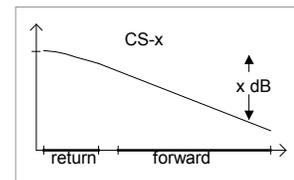
**Return Path Attenuation (RA):** The return path attenuator is used in systems deploying high-speed data services that are utilizing the return path. The return path attenuator is normally used in low value taps toward the end of the distribution system that have low loss in the return path. The advantages of the return path attenuator are:
