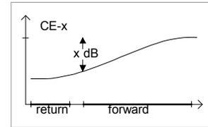
**Cable Simulator (CS):** The cable simulator is used in the latest system designs that incorporate high output amplifiers allowing the full use of the amplifier gain and large positive tilts. The cable simulator is normally used in the first few taps after an amplifier. The advantages of the cable simulator are:
