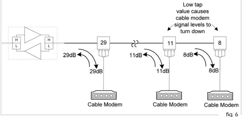
Conventional Distribution System Using Cable Modems With E-Option Return Path Attenuation
